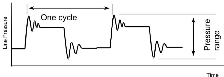
**Figure 1 : Pressure Cycle**
