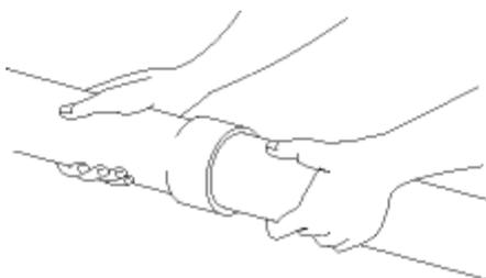
Hold the joint against movement and rejection (i.e. pushback) of the spigot for a minimum of 30 seconds.
