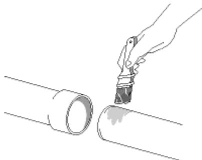
Using a suitably sized brush, apply a thin even coat of solvent cement to the internal surface of the socket first. Solvents will evaporate faster from the exposed spigot than from the socket. Special care should be taken to ensure that excess solvent cement isn't built up at the back of the socket (pools of solvent will continue to attack the PVC and weaken the pipe). Next apply a similar even coat of solvent cement up to the witness mark on the spigot. Ensure the entire surface is covered.
