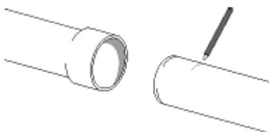
It is essential to be able to determine when the spigot is fully home in the socket. Mark the spigot with a pencil line ('witness mark') at a distance equal to the internal depth of the socket.
