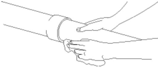
For a neat professional joint, with a clean rag, immediately wipe off excess solvent cement from the outside of the joint.
