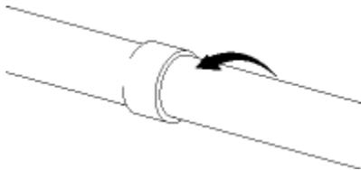
Make the joint immediately, in a single movement. Do not stop halfway, since the bond will start to set immediately and it will be almost impossible to insert further.
