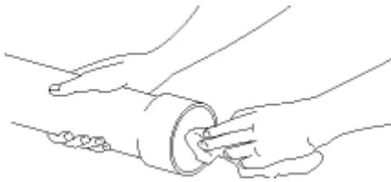
Priming is vitally important, as it cleans and primes the PVC surface for the solvent cement's effective bond.
